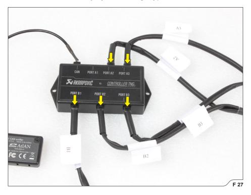
3. Carefully separate the **brown-orange** and **black-orange** wires from the stock harness, unscrew the CAN sniffer's cover, lead the **brown-orange** and **black-orange** wires through the CAN sniffer's wire grooves as shown, reinstall the cover and secure the TNG controller in place, using tie wraps from Akrapovič installation kit (**F 28, 29, 30**).
