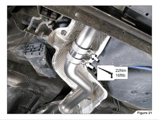
12. For Slip-On only: push the middle and muffler inlet pipe together and tighten the clamps to the specified torque (Figure 22).
