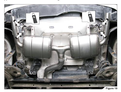
For Slip-On and Evolution: center the muffler-height wise. The muffler's outlets on both sides of the vehicle must be equally distanced from the chassis (Figure 20).
