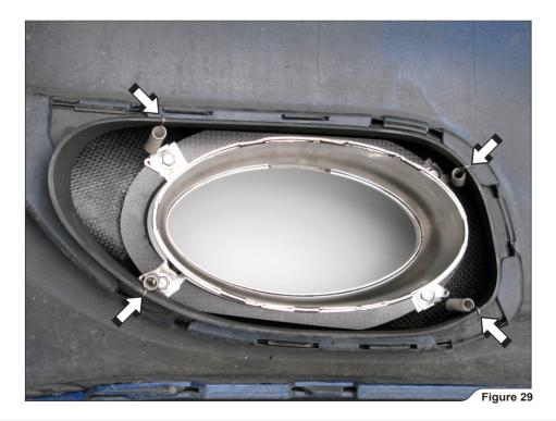
15. For Slip-On and Slip-On with optional Link Pipes: replace the dismounted stock muffler heatshield and rear bumper in the reverse order from the order in which they were removed. Check vehicle manufacturer manual for tightening torques (Figure 30).
