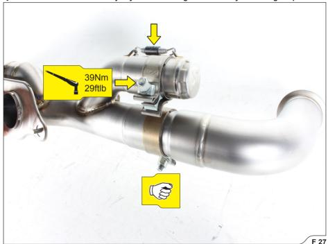
8. For Slip-On Race only: install the Slip-On Race system onto the vehicle and hand tighten Akrapovič clamps (F 28, 29).
