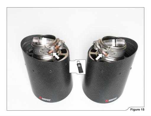
10. **For Slip-On and Evolution:** slide the tail-pipes onto the muffler outlets. Rotate and center them in respect to rear bumper as shown **(Figure 16, 17, 18).**
