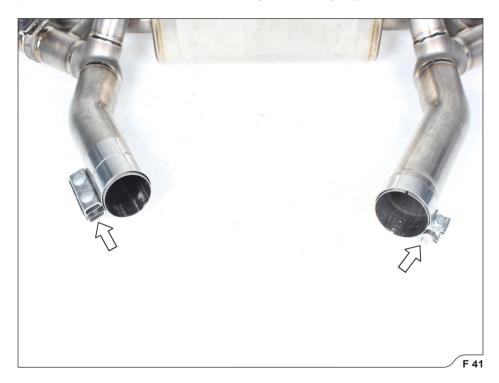
! IMPORTANT: unscrew the double clamp's nuts enough, to be able to slide the clamp completely onto the pipe (F 42)!
