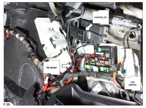
Carefully separate the yellow-brown and yellow-red wires from the stock harness (at the right side of the fuse box), unscrew the CAN sniffer's cover, lead the yellow-brown and yellow-red wires through the CAN sniffer's wire grooves as shown, reinstall the cover and secure the CAN sniffer's cable, using tie wrap from Akrapovič installation kit (F 21, 22).
