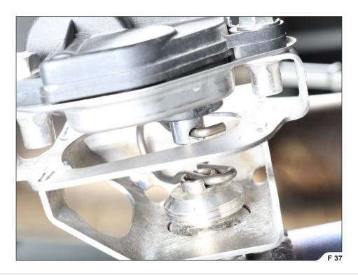
! IMPORTANT: DUE TO A DELIBERATE PRE-TENSION OF THE VALVE, THE STOCK C-SPRING NEEDS TO BE TENSIONED DURING ACTUATOR INSTALLATION (IN OTHER WORDS, THE VALVE ACTUATOR NEEDS TO BE ROTATED, SO THE C-SPRING IS TENSIONED, UNTIL THE ACTUATOR'S BOLT HOLES ALIGN WITH THE VALVE'S THREADED BOLT HOLES)!
