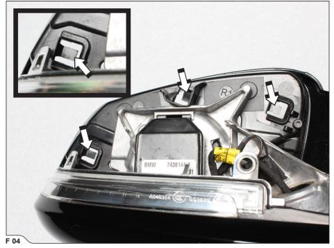
2. Correctly position and install Akrapovič mirror cover cap onto the exterior mirror (F 05).
