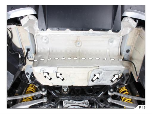
7. Connect Akrapovič cable set to the stock connector and protect the cables using tie wraps from Akrapovič installation kit (F 14).
