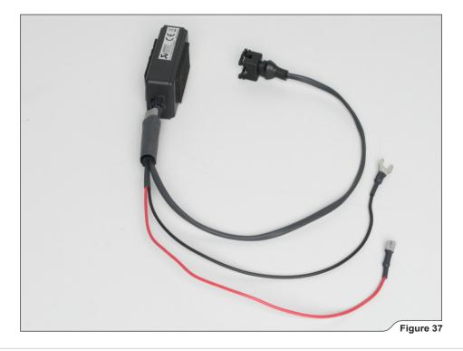
10. Place the transmitter in the right side of the car boot (behind the boot panel). Tighten the ground connector (black thin wire) with marked nut, install the connector (black thick wire with connector) to the electromagnet valve and install the fuse box connector (red wire) in the marked spot in the fuse box (Figure 38, 39, 40).
