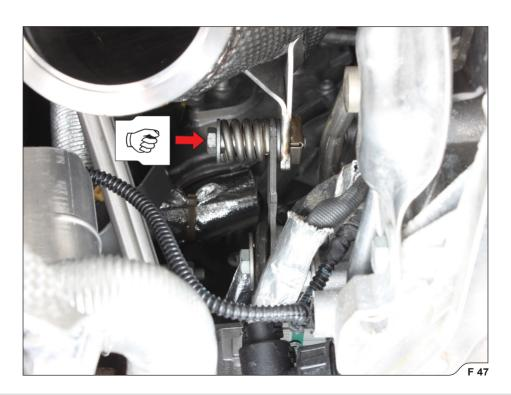
In case of the gap between the Downpipes' bracket and stock bracket: hand tighten the Downpipes' brackets, using stock springs and bolts and washers from Akrapovič installation kit; in respect to the gap, use one or two washers (F 48, 49, 50).
