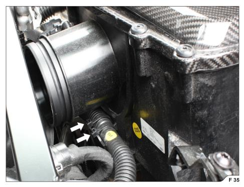
IMPORTANT: before removing the left air-box, cut the marked tie wraps (F 35)!
